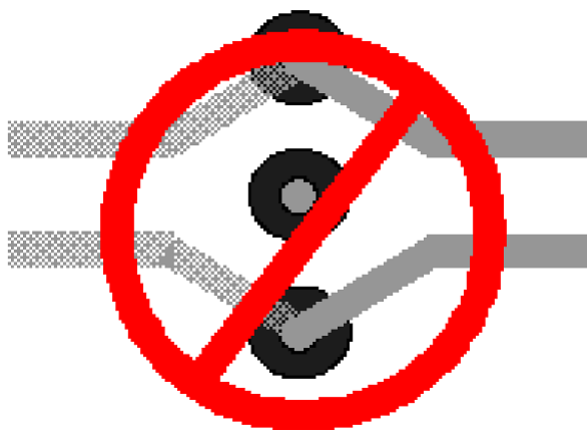
Figure 8-4. No Vias Between High-Speed Traces
